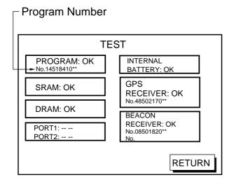
Figure 12-21 Memory, I/O test results
